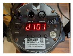
The Performer 18 has two DMX modes. We recommend 8-channel mode. Press Menu until the display says **8Ch** and confirm your choice by pressing Enter.
